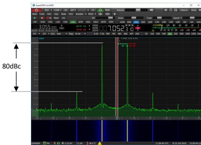
P_i=2x-20dBm , Bandpass-Filter On, IMD3=80dBc ID3 > 20dB above noise (this is too much)
