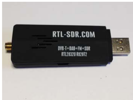
Bild 1: "RTL-SDR.COM", DVBT-Stick RTL2832U R820T2 TCXO, 24 – 1766MHz
